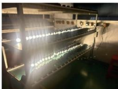
Aging Test Area
