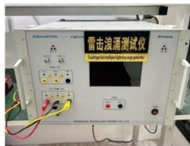
Lightning Surge Generator
